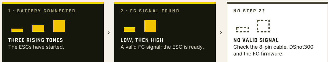
FIG-38 Start-up sequence heard through the motors (props off). Bar height shows the relative pitch of each tone.
