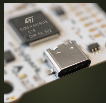
FIG-51 All flashing is done over the USB-C port. Use a data cable, not a charge-only cable.
