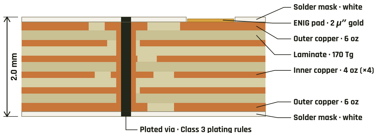
FIG-08 Illustrative cross-section of the 6-layer V2 ESC power board. Diagram, not to scale.
